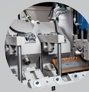
VP-X 166 with separate one-piece units with short punches
