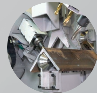
Drill units above the angle: easy collection of chips and coolant
